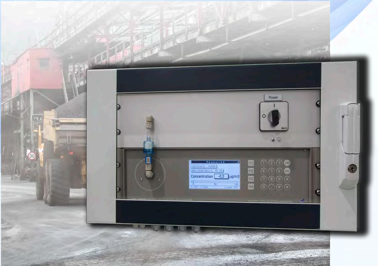
All necessary cables and tubings are fed through the dustproof cable glands on the bottom of the enclosure. The VM-3000 unit has all of its electrical in- and outputs as well as the sample gas in- and outlet on the rear. They are easily accessible by simply swinging open the enclosure.
